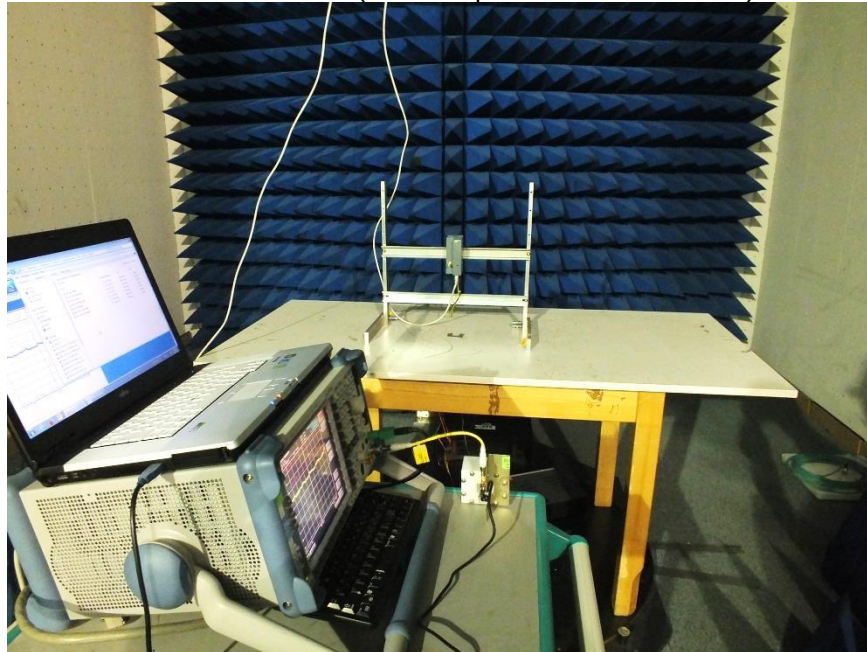
Anechoic chamber (Test setup for 18 GHz – 40 GHz)
