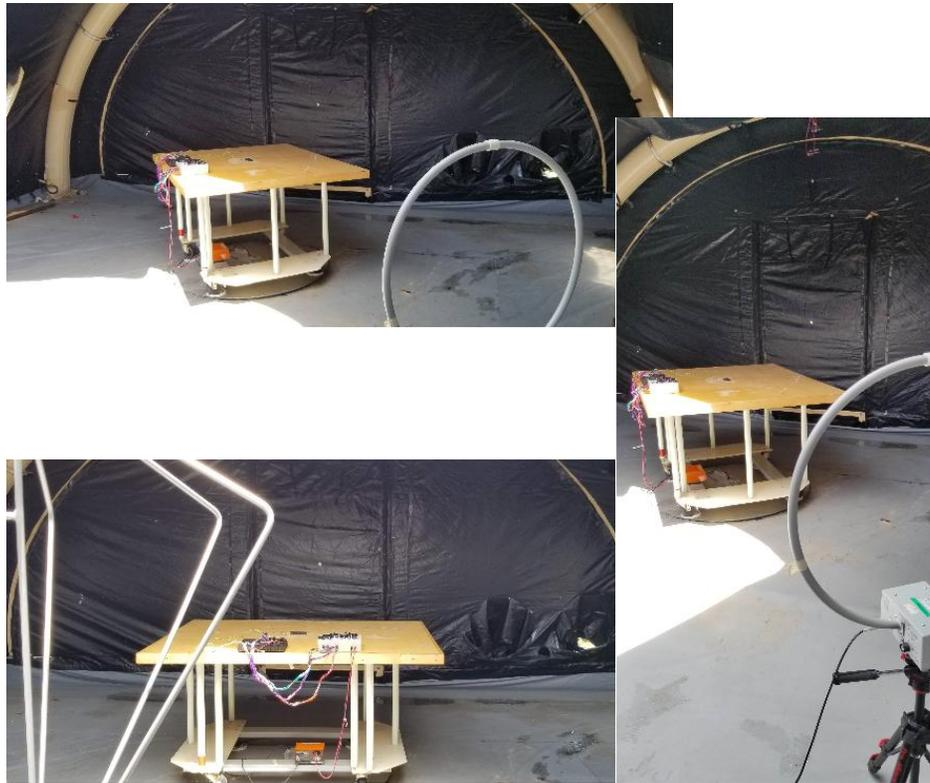
Figure 4: Radiated Emissions Test Setup Photograph(s).
