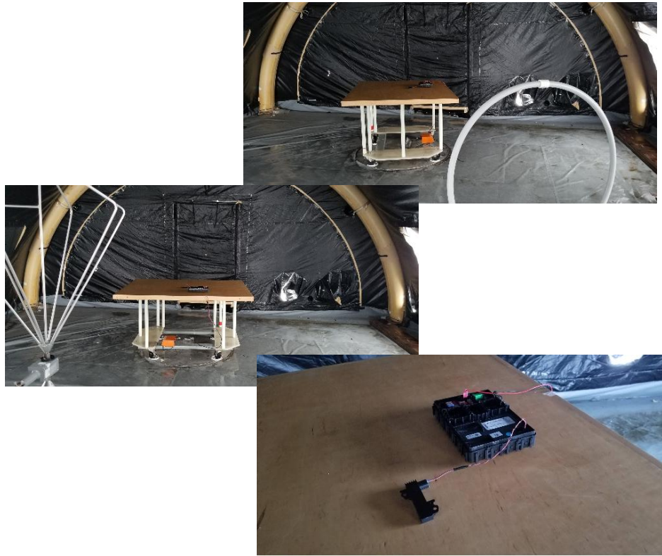
Figure 4: Radiated Emissions Test Setup Photograph(s).
