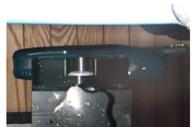
Figure 16. Body SAR Test Setup without Belt Clip
