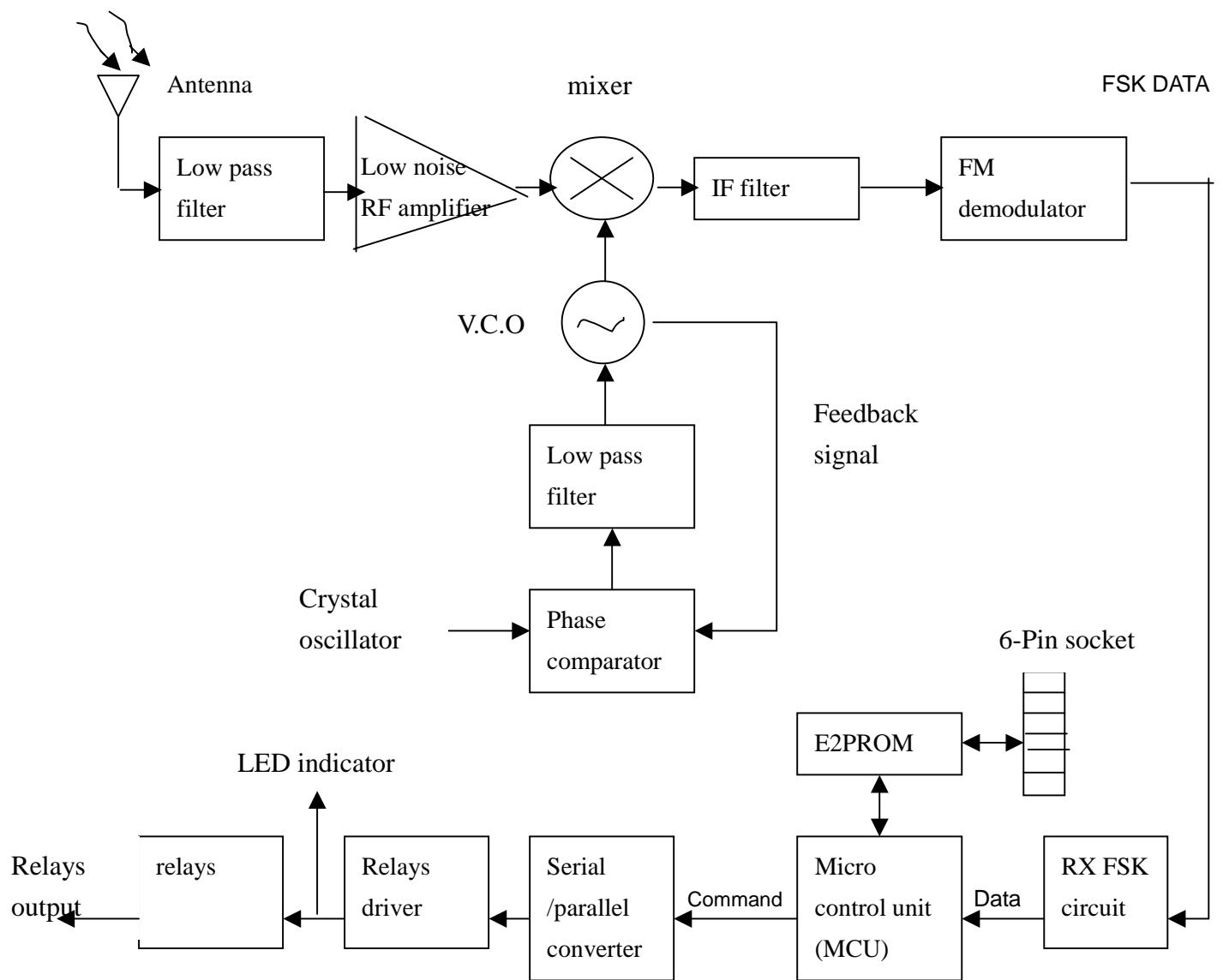
Fig.2 Receiver's function block diagram
