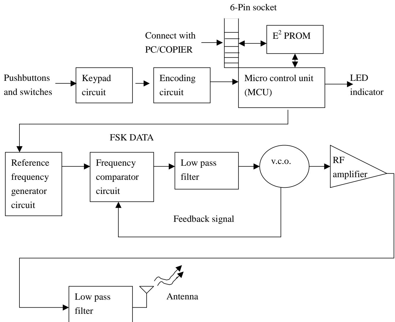
Fig.1 Transmitter's function block diagram
