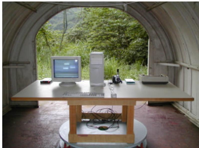
Radiated Emission Setup Photos (Worst Emission Position)
