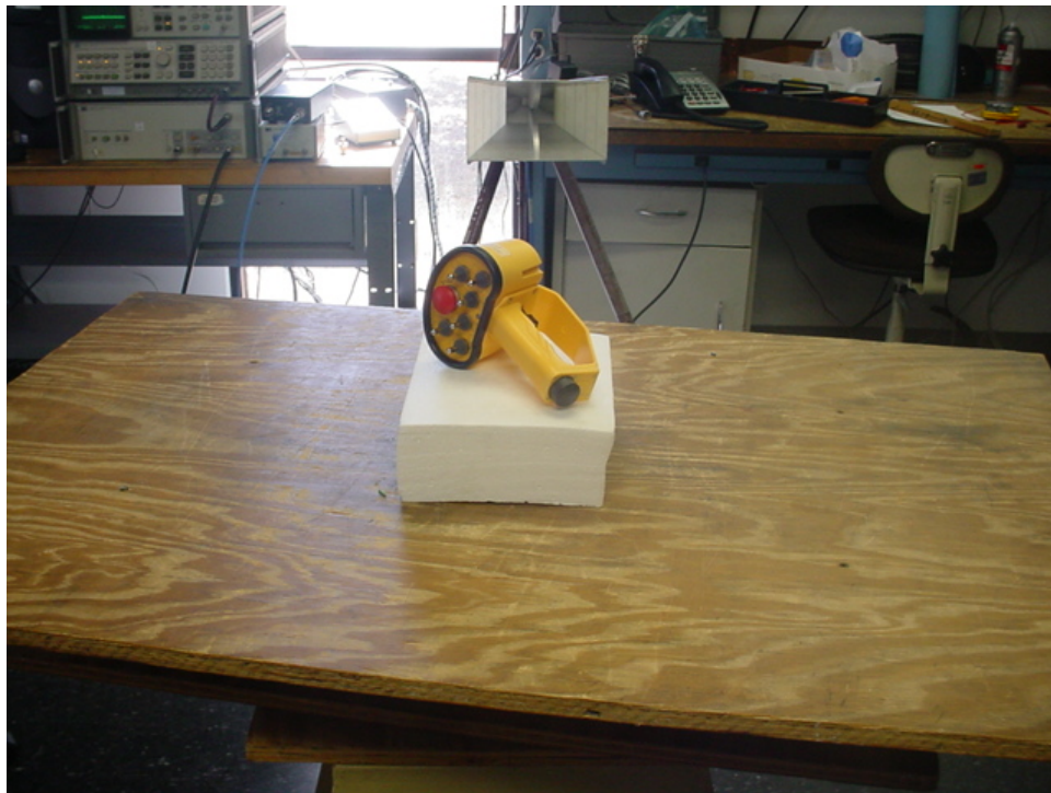
Microwave Radiated Emission Test Setup
