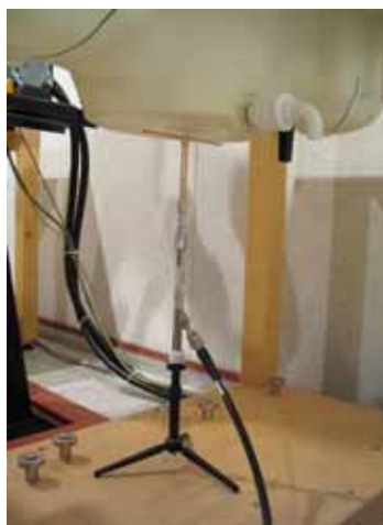
Photo of the dipole Antenna
