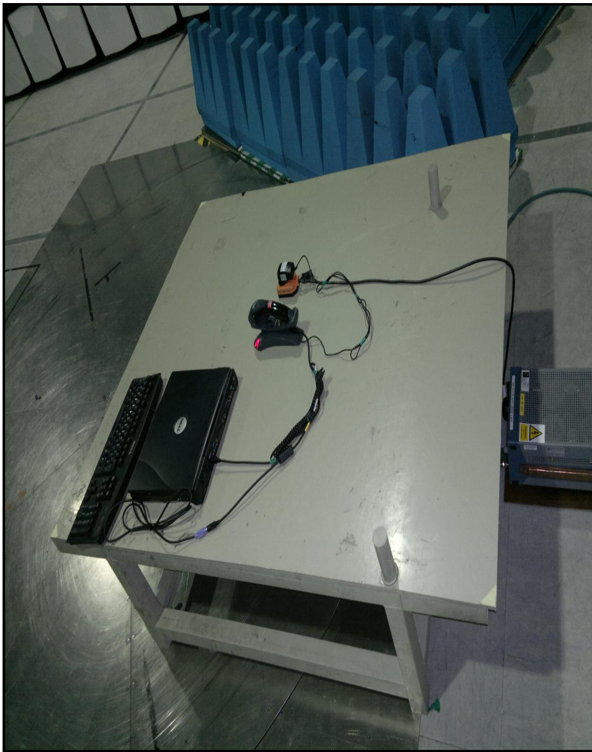
**PHT\83519JD04\002 - Test Configuration Photograph - Radiated Emissions**
