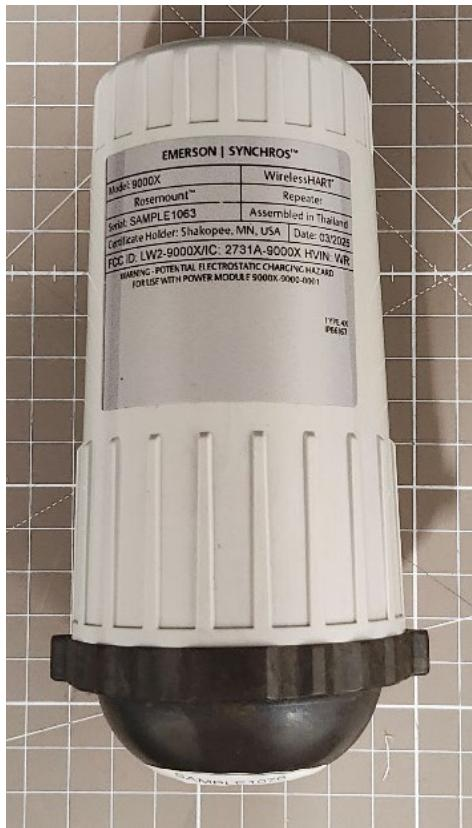
The FCC ID will be printed on a thermal transfer polyester label permanently adhered to the exterior of the device in the location shown in the images shown here.
