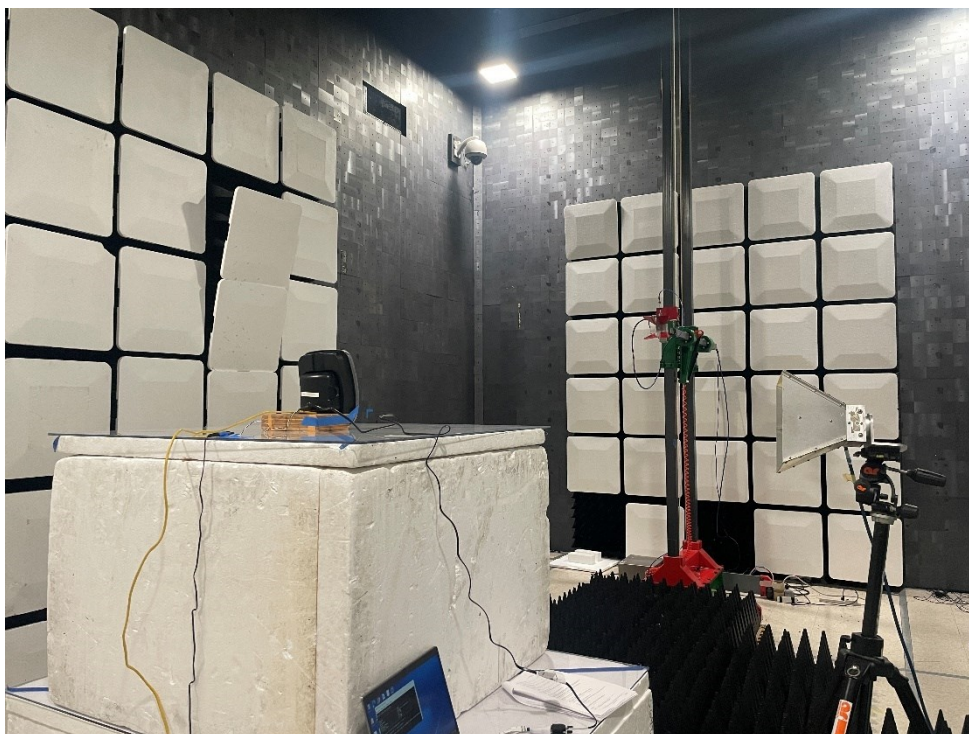
Figure 8.1.11 Radiated emissions 1-18 GHz (Back)
