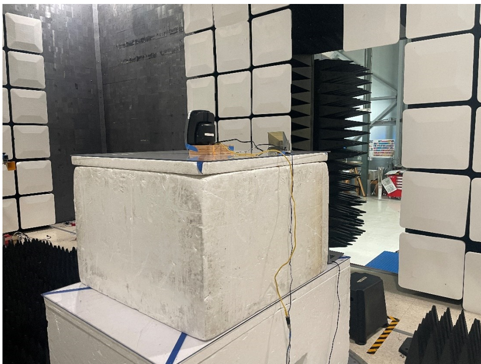
Figure 8.1.13 Radiated emissions 18-26.5 GHz (Back)
