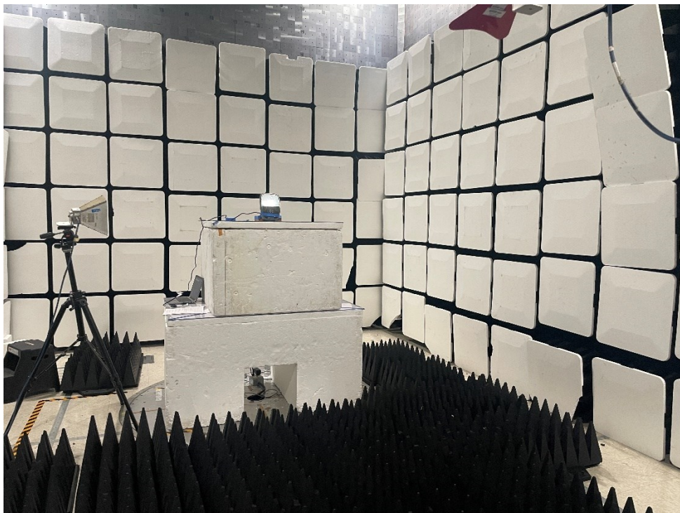
Figure 8.1.10 Radiated emissions 1-18 GHz (Front)
