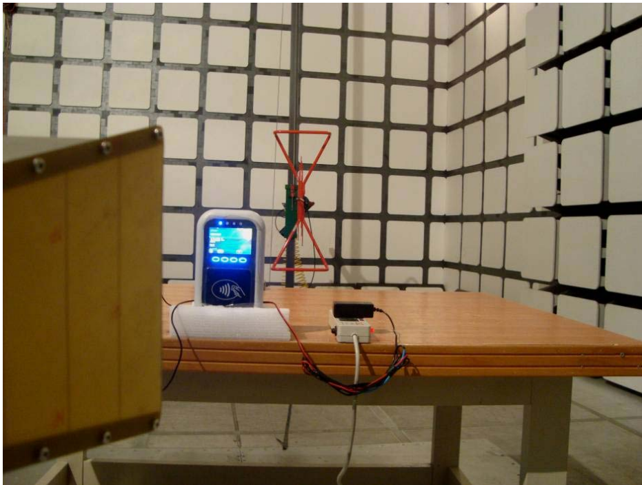
Below 1 GHz: Radiated Emissions - Rear View
