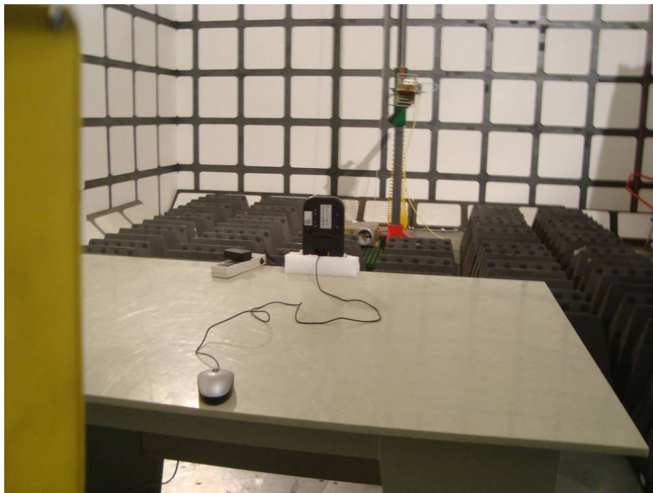
Above 1 GHz: Radiated Emissions - Rear View
