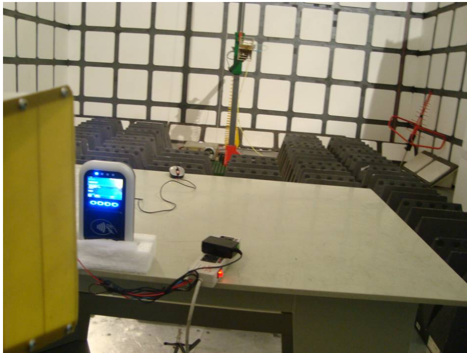
Above 1 GHz: Radiated Emissions - Rear View
