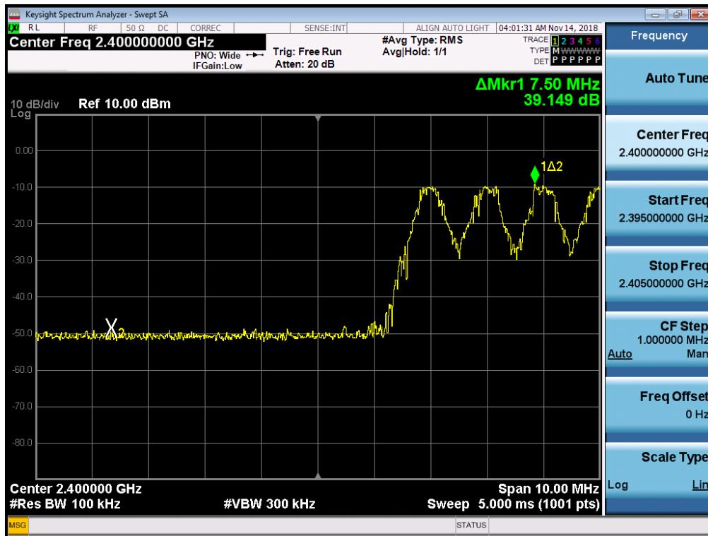
Test Plots with hopping (GFSK)
