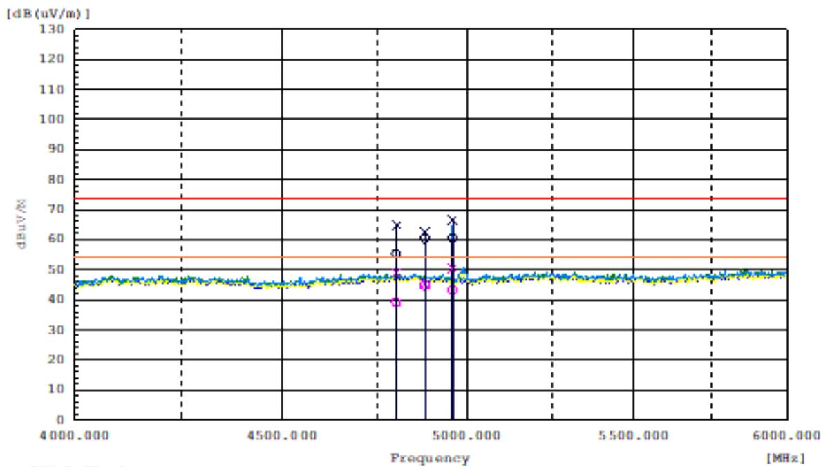
**Radiated Spurious Emissions plot – (S740\_ Battery Mode GFSK, 2nd Harmonic)**
