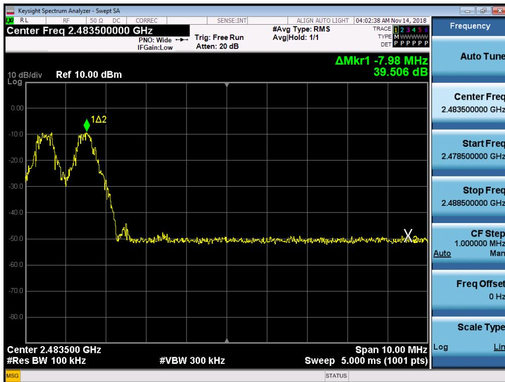
Test Plots with hopping (8DPSK)
