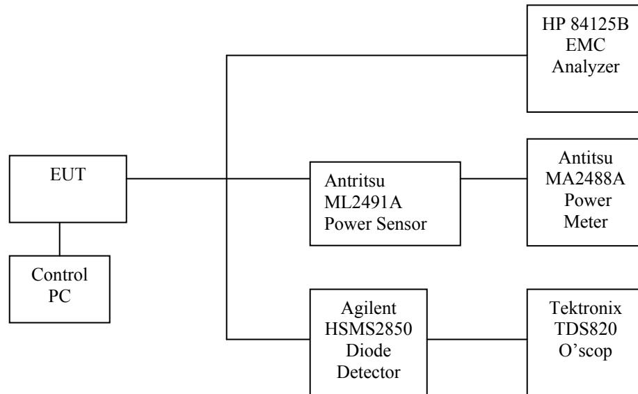
The solid lines are coaxial cables and the dashed lines are either EUT insertion to the test board or control cables between test setup devices. The measurement results were adjusted with the attenuation of the coaxial cable.
