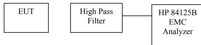
Note: The high –pass filter is used for the Radiated Spurious emissions above 2.4835 GHz. A pass-thru connector is used for Radiated Spurious emissions measurements from 30 MHz – 2.4 GHz.
