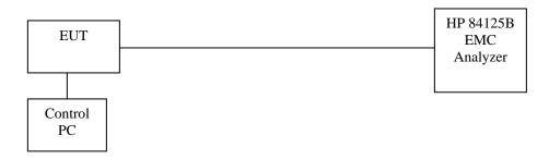
The solid lines are coaxial cables and the dashed lines are either EUT insertion to the test board or control cables between test setup devices. The measurement results were adjusted with the attenuation of the coaxial cable.
