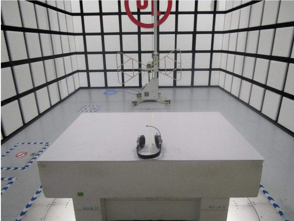
Radiated Disturbance below 30 MHz
