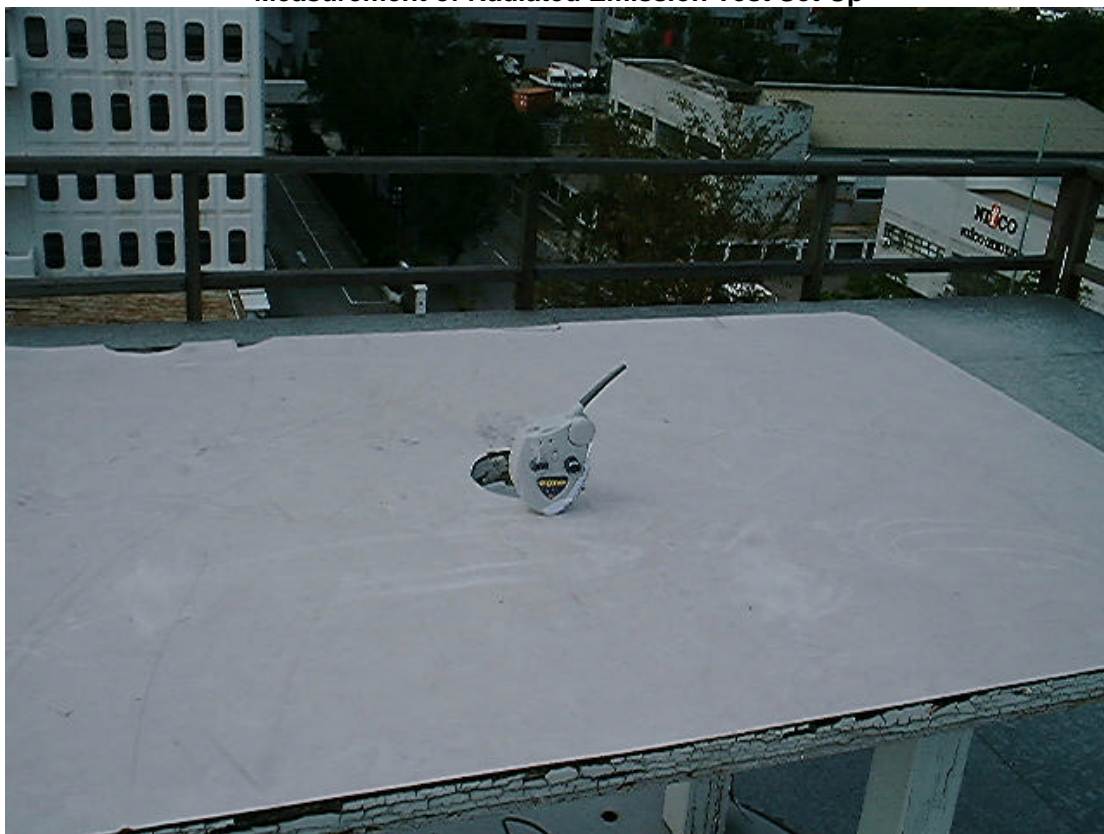
Measurement of Radiated Emission Test Set Up
