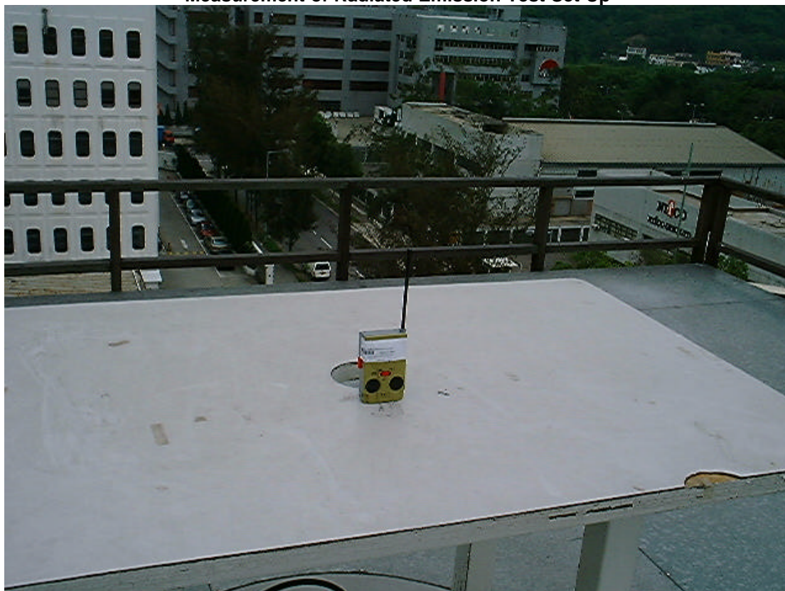
Measurement of Radiated Emission Test Set Up
