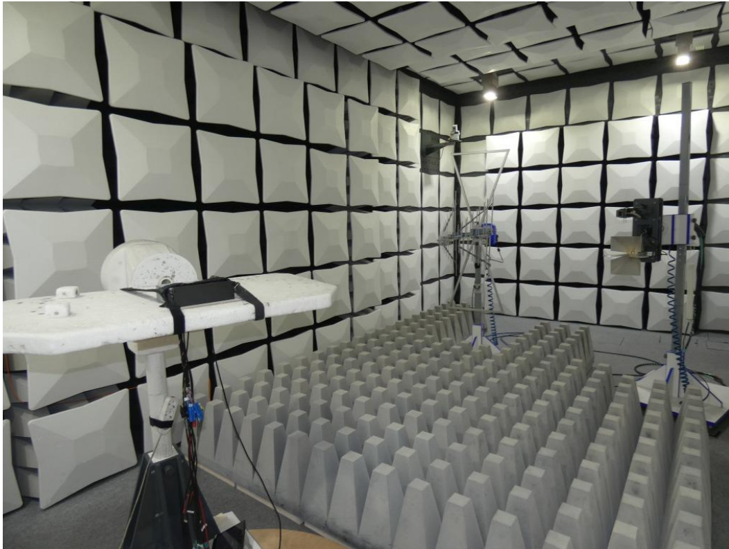
Photo 3: Test setup for radiated measurements above 1 GHz
