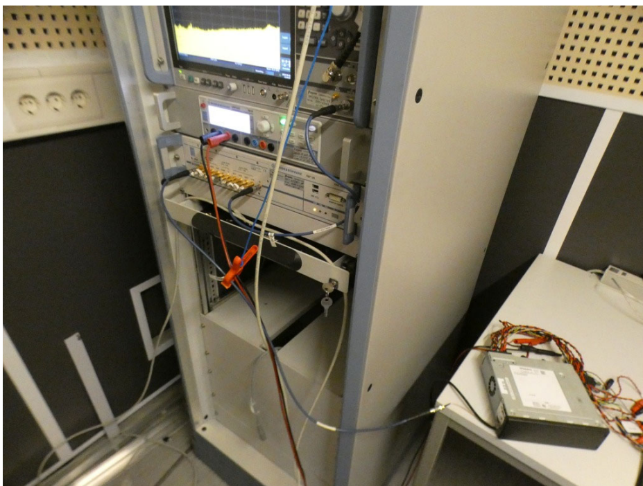
Photo 2: Test setup for Conducted measurements FCC15.247
