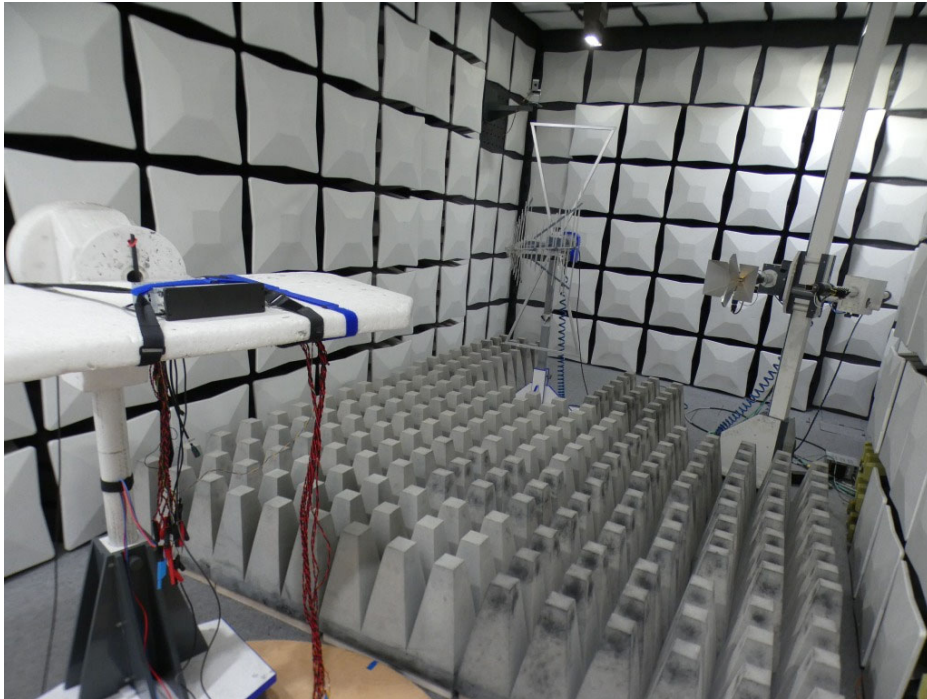
Photo 1: Test setup for radiated measurements above 1 GHz
