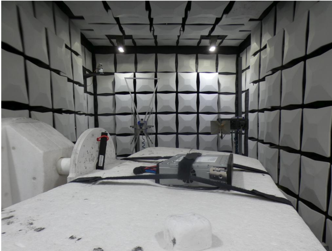
Photo 3: Test setup for radiated measurements above 1 GHz
