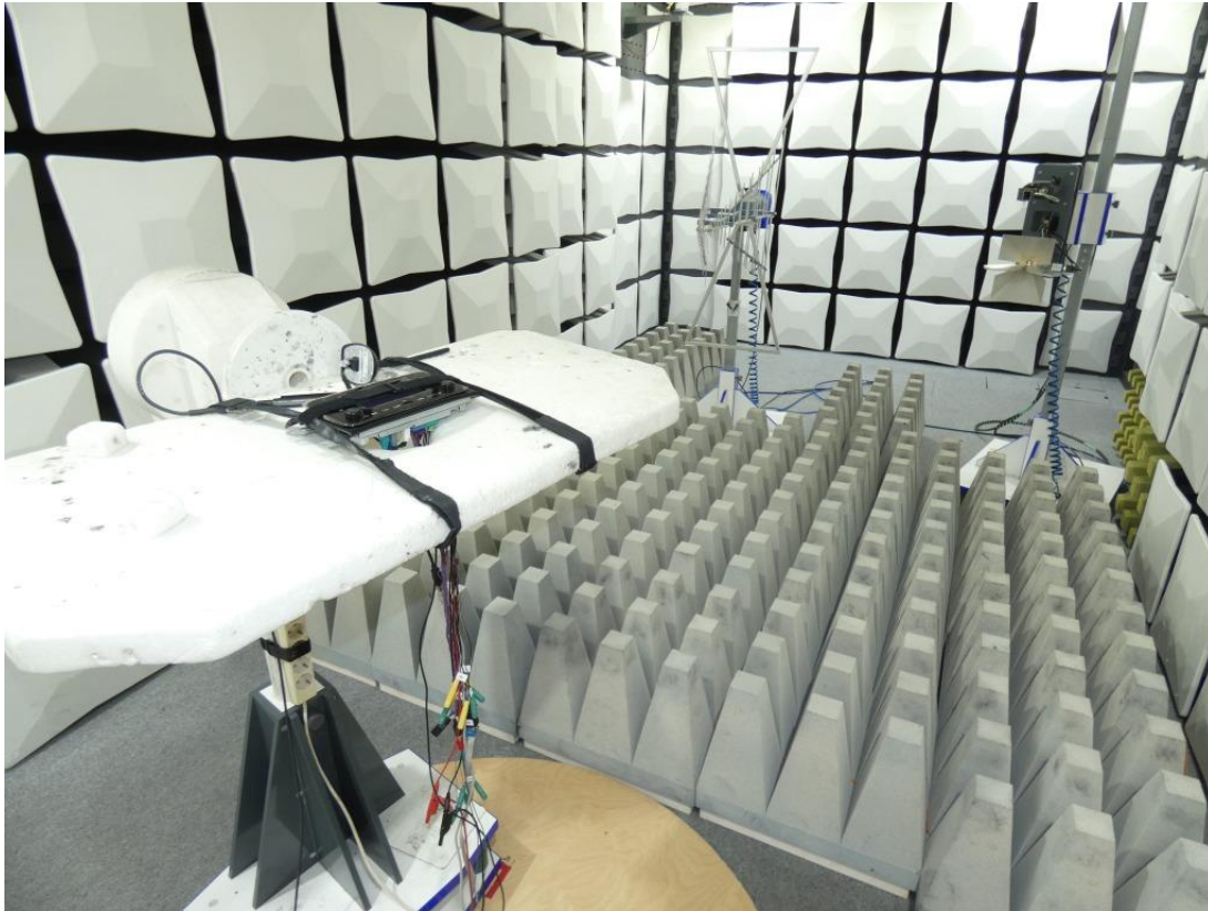
Photo 3: Test setup for radiated measurements (1 GHz – 26 GHz; FCC 15c247)
