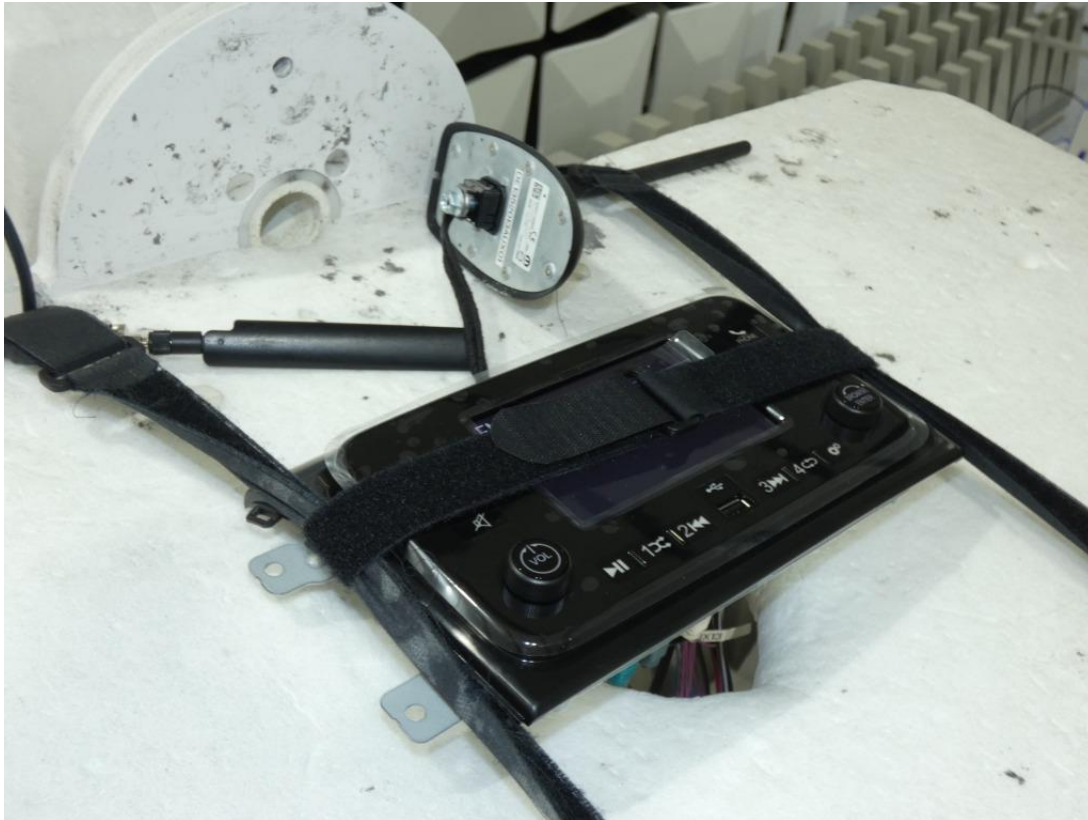
Photo 4: Test setup for radiated measurements, EUT
