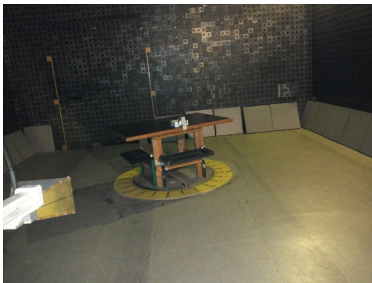
Photograph 8.1.2 Setup for radiated emission measurements
