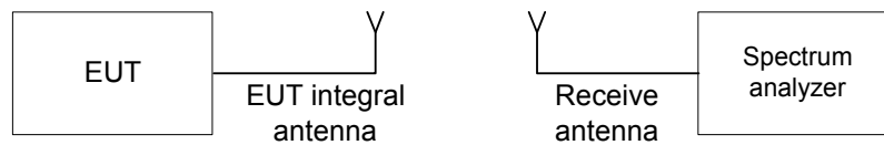
Figure 7.1.1 Setup for transmitter shut down test
