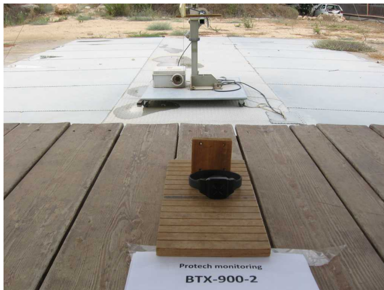
Figure 4. Radiated Emission Test Above 1 GHz
