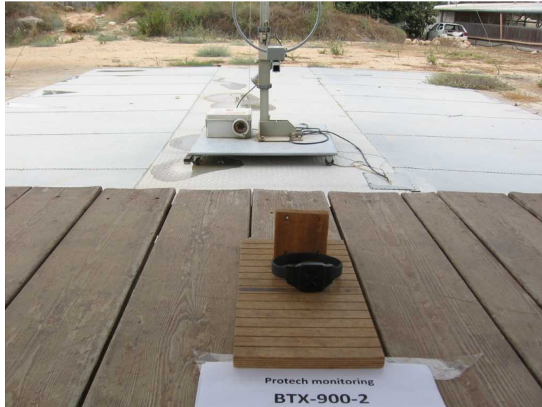
Figure 2. Radiated Emission Test 9 kHz – 30 MHz
