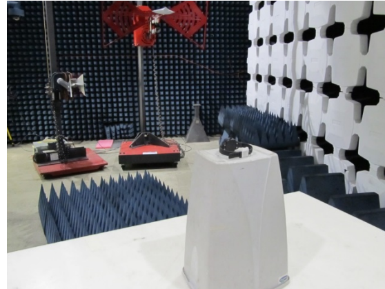
Radiated emissions test set up above 1GHz.
