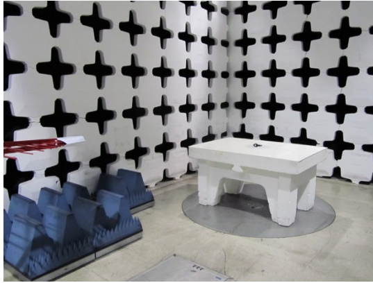
Radiated emissions test set up below 1GHz.
