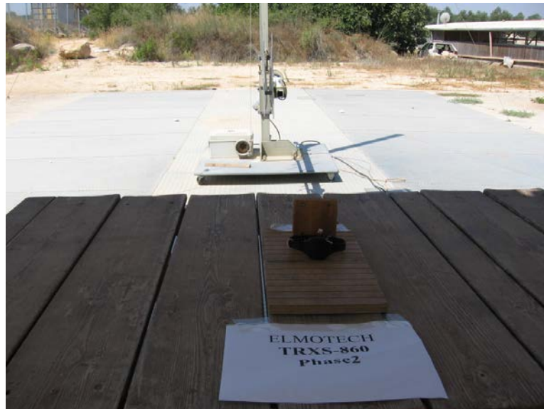
Figure 2. Radiated Emission Test 30 MHz – 1000 MHz
