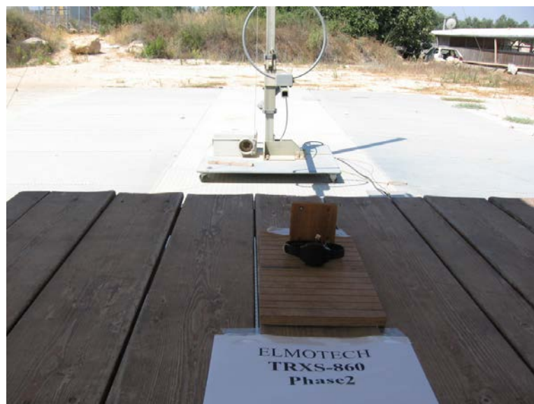
Figure 3. Radiated Emission Test 9 kHz – 30 MHz
