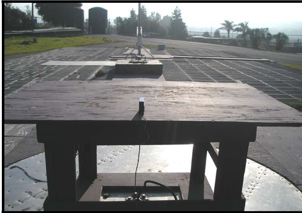
Figure 1: Open Field Radiated Emissions below 1 GHz (View 1)
