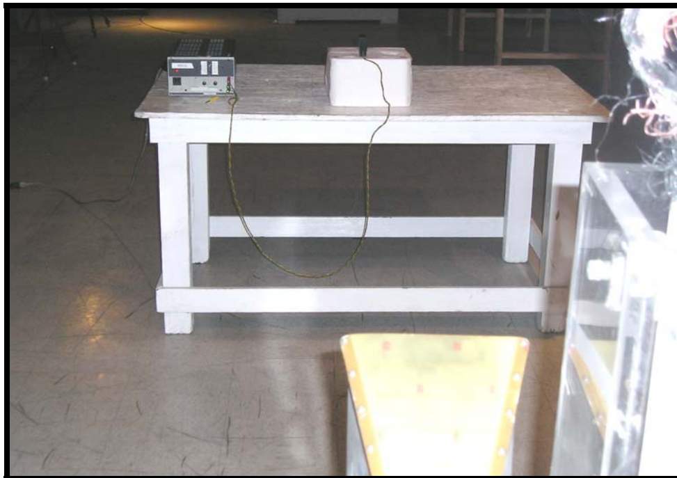
Figure 8: Spurious emission above 1 GHz (View 2)
