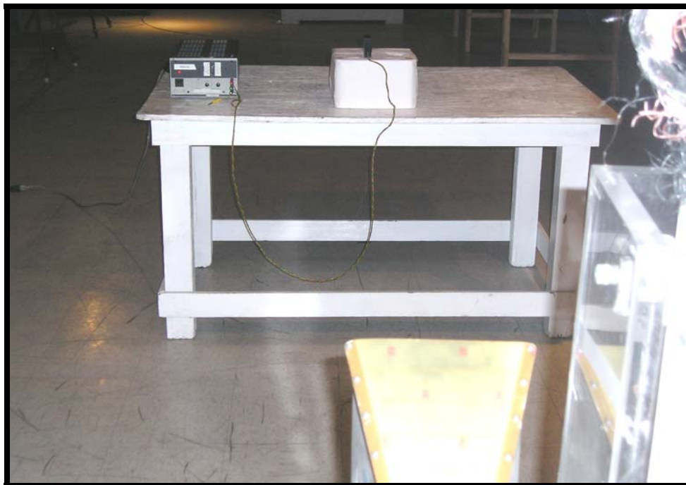
Figure 4: Radiated Emissions above 1 GHz (View 2)
