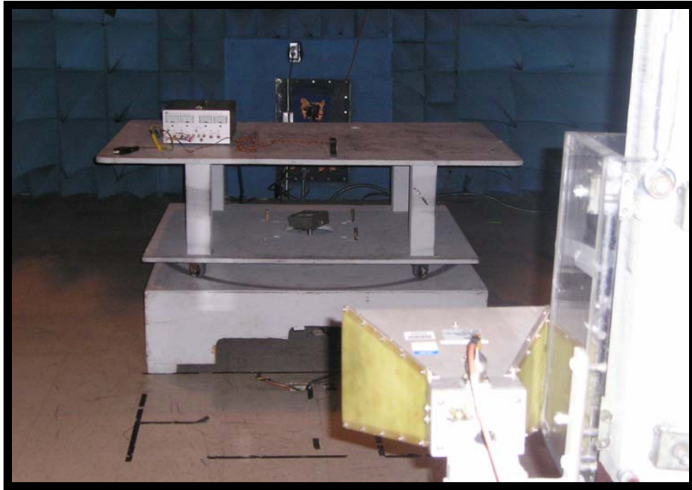
Figure 5 Field Strength of Fundamental Measurement (Front)
