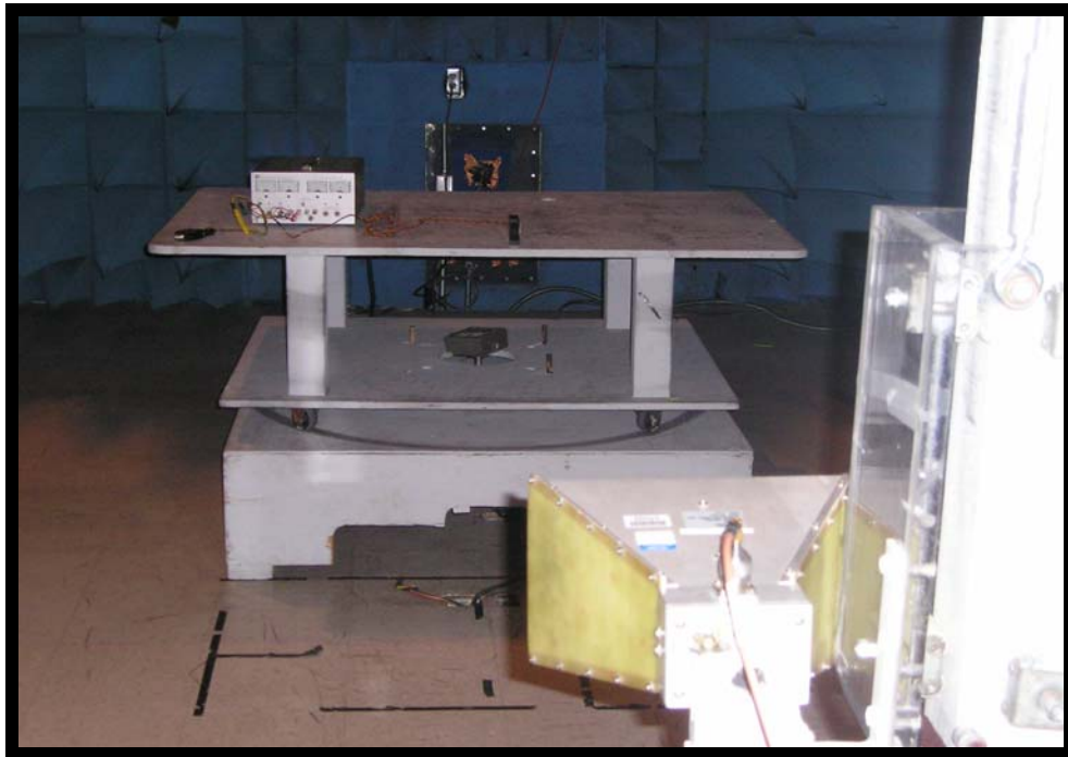
Figure 3: Radiated Emissions above 1 GHz (front view)
