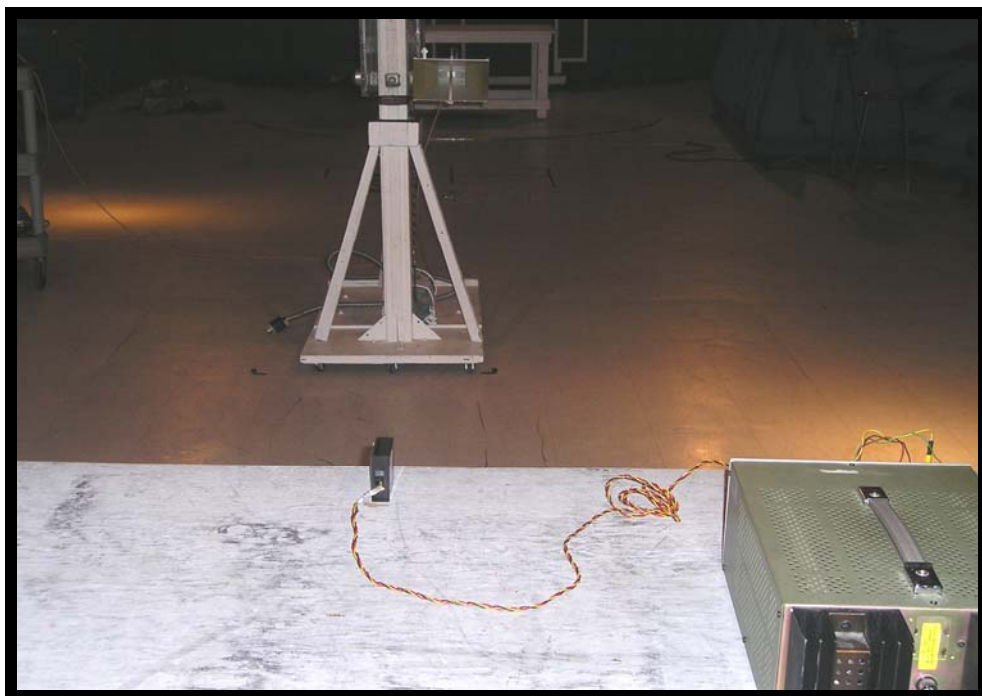
Figure 4: Radiated Emissions above 1 GHz (rear view)
