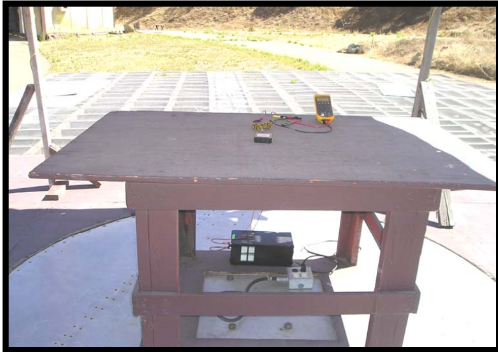
Figure 7: Spurious emissions below 1 GHz (front view)
