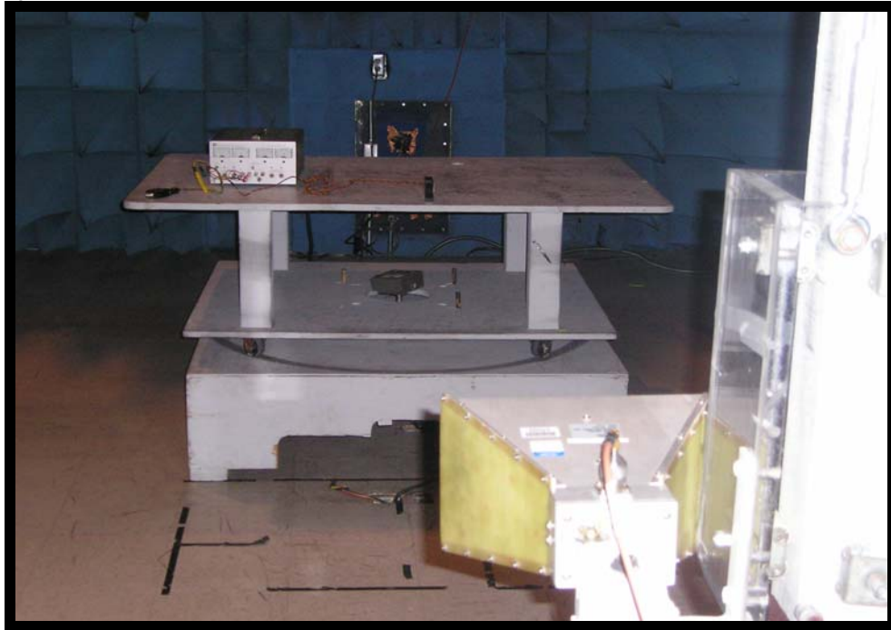
Figure 9: Spurious emission above 1 GHz (front view)
