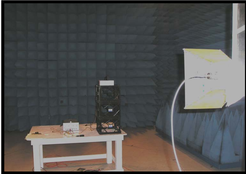
Figure 3: Radiated Emissions above 1 GHz (front view)
