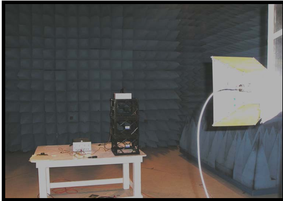
Figure 9: Spurious emission above 1 GHz (front view)
