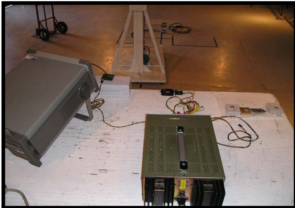
Figure 6 Test Set Up Photos – Field Strength of Fundamental Measurement (Rear)
