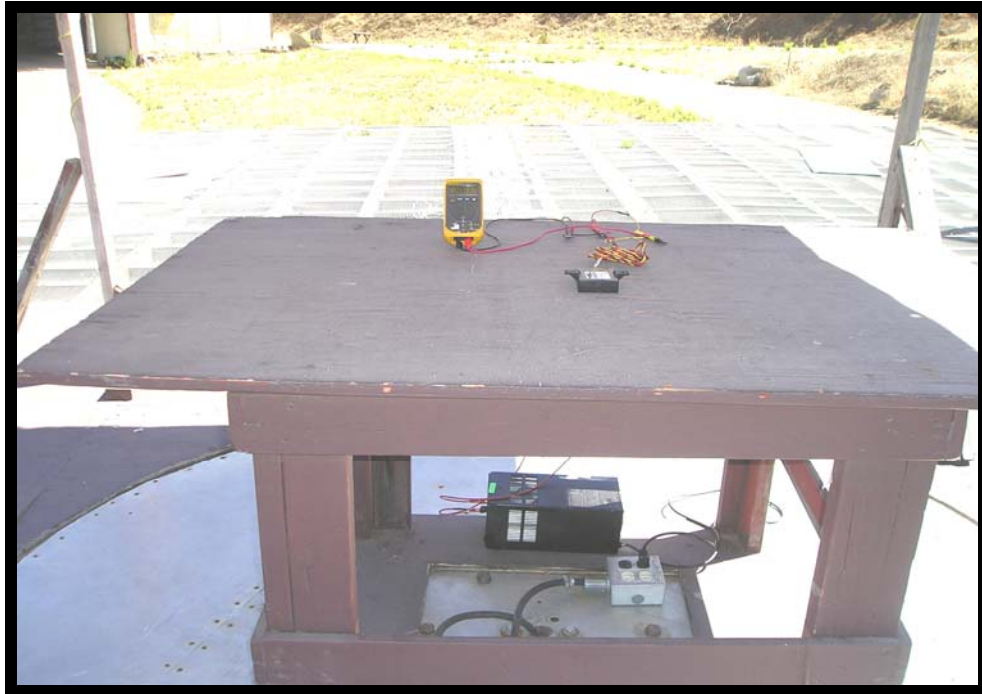
Figure 1: Open Field Radiated Emissions Test Setup below 1 GHz (front view)
