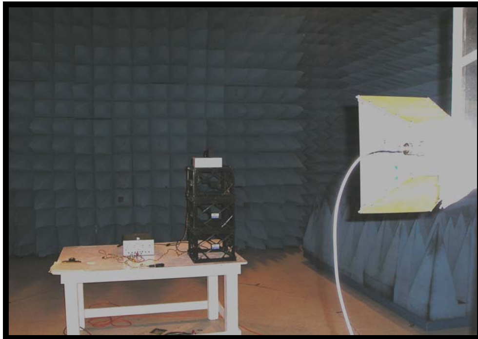
Figure 3: Radiated Emissions Test Setup, above 1 GHz (front view)
