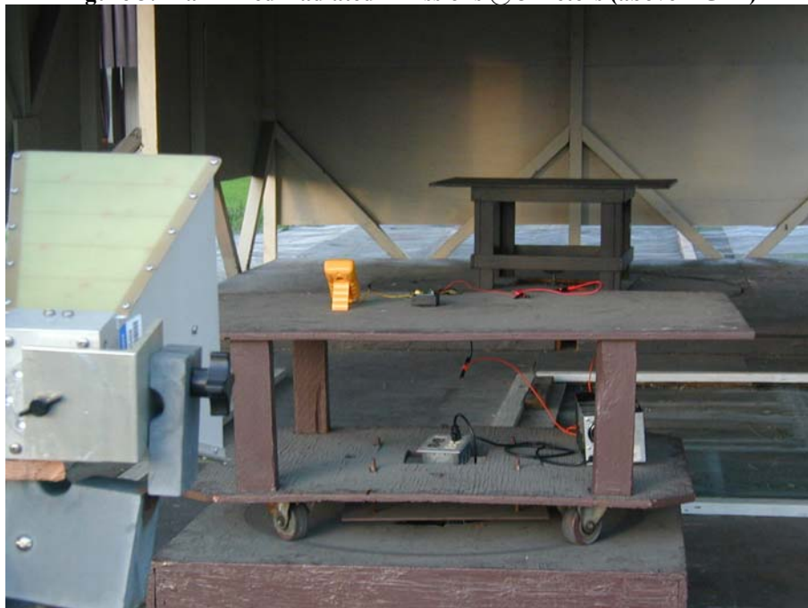
Figure 4: Maximized Radiated Emissions @ 3 meters (above 1 GHz)
