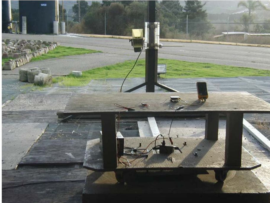
Figure 3: Maximized Radiated Emissions @ 3 meters (above 1 GHz)
