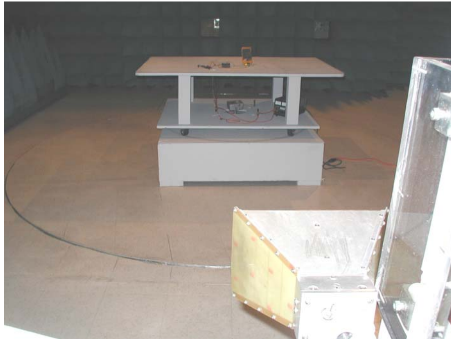
Figure 5 Test Set Up Photos – Field Strength of Fundamental Measurement (Front)
