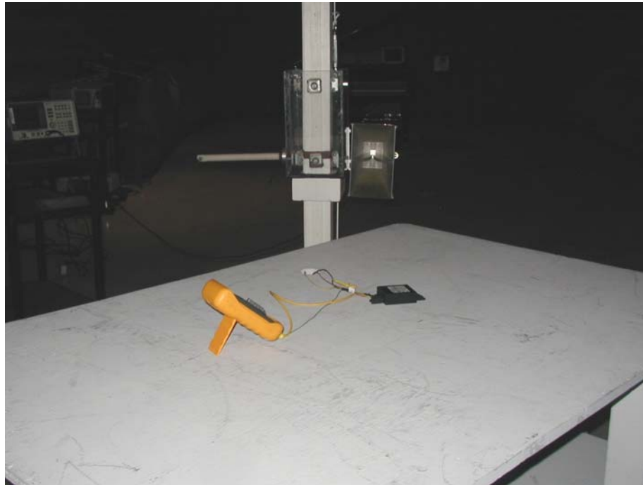
Figure 7 Test Set Up Photos – Spurious, Harmonics, and Restricted Bands Test Setup @ 1 meter (above 18GHz)
