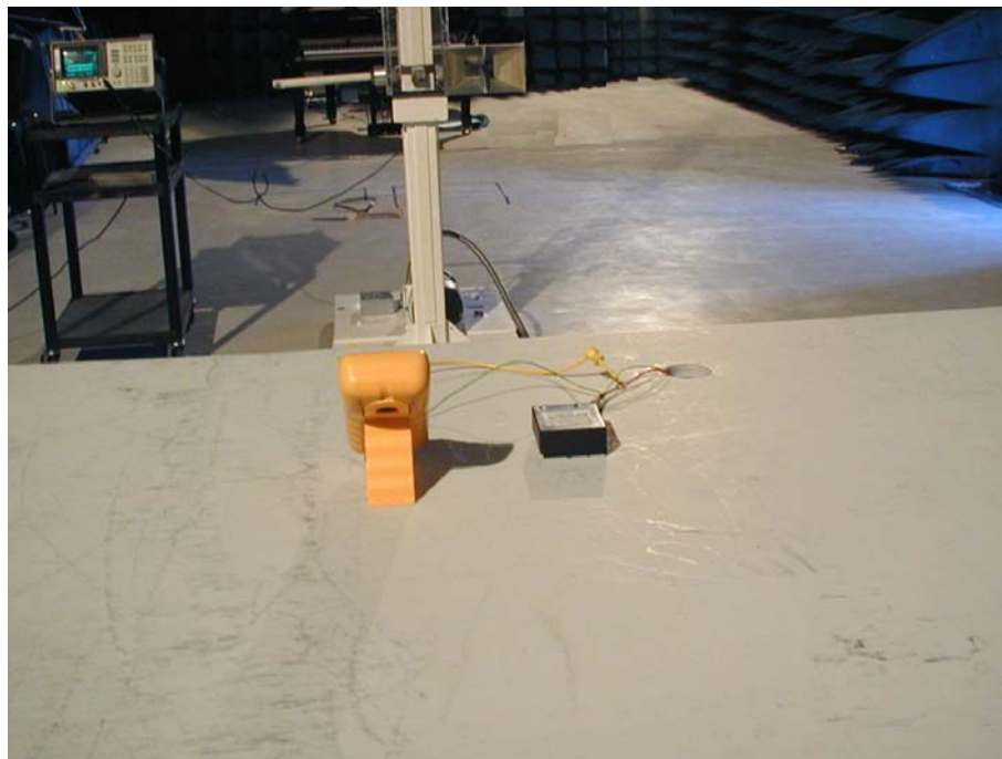
Figure 6 Test Set Up Photos – Field Strength of Fundamental Measurement (Rear)
