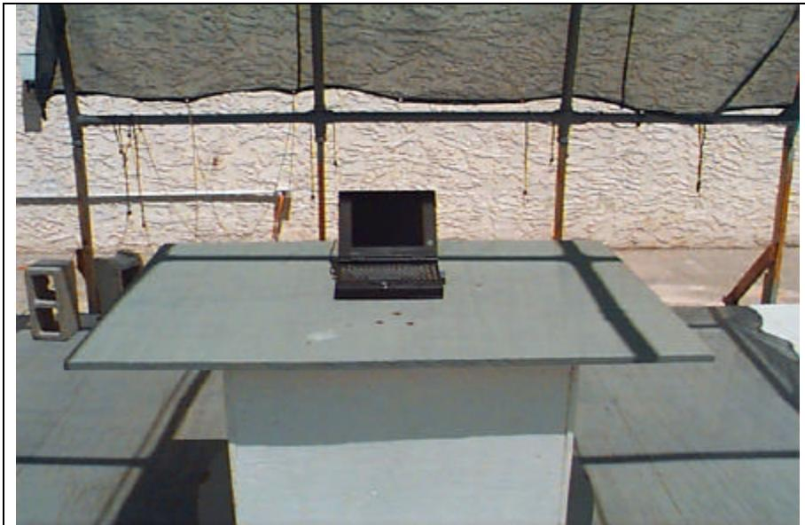
TEST SETUP: Radiated Emissions
