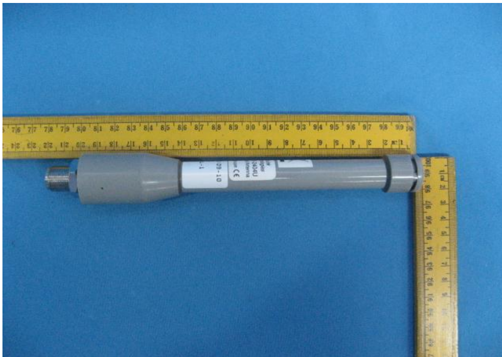
Antenna 1 – Dimensional View
