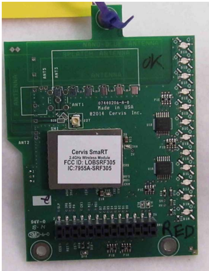
Figure 5. 07440306-2H-U-12R, SRF305 Type 3,, component side, shield and internal label, external antenna connector
