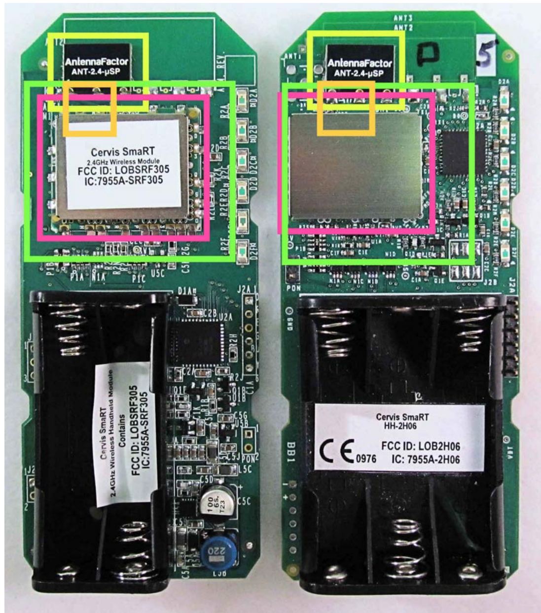
Figure 7. HH-2H10 (left) implemented with Type 4 module, compared to HH-2H06 with non-modular RF circuit integrated into the application PCB. In both applications the RF circuit under the shield is identical.
