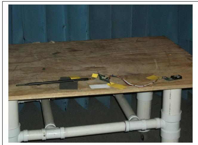
**Radiated Spurious Emission with 9dBi Whip Antenna: OATS**
