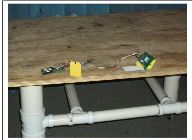
**Radiated Spurious Emission with 3.8dBi Integral Antenna: OATS**
