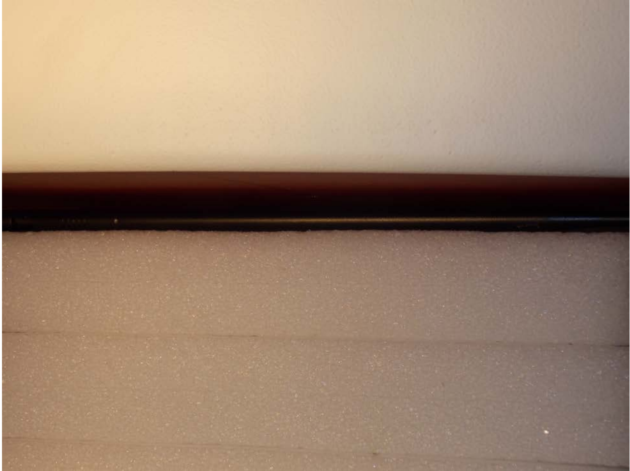
Test Position External Antenna 8 mm Gap Testing Conducted at 0°, 60°, 120°, 180°, 240° and 300°
