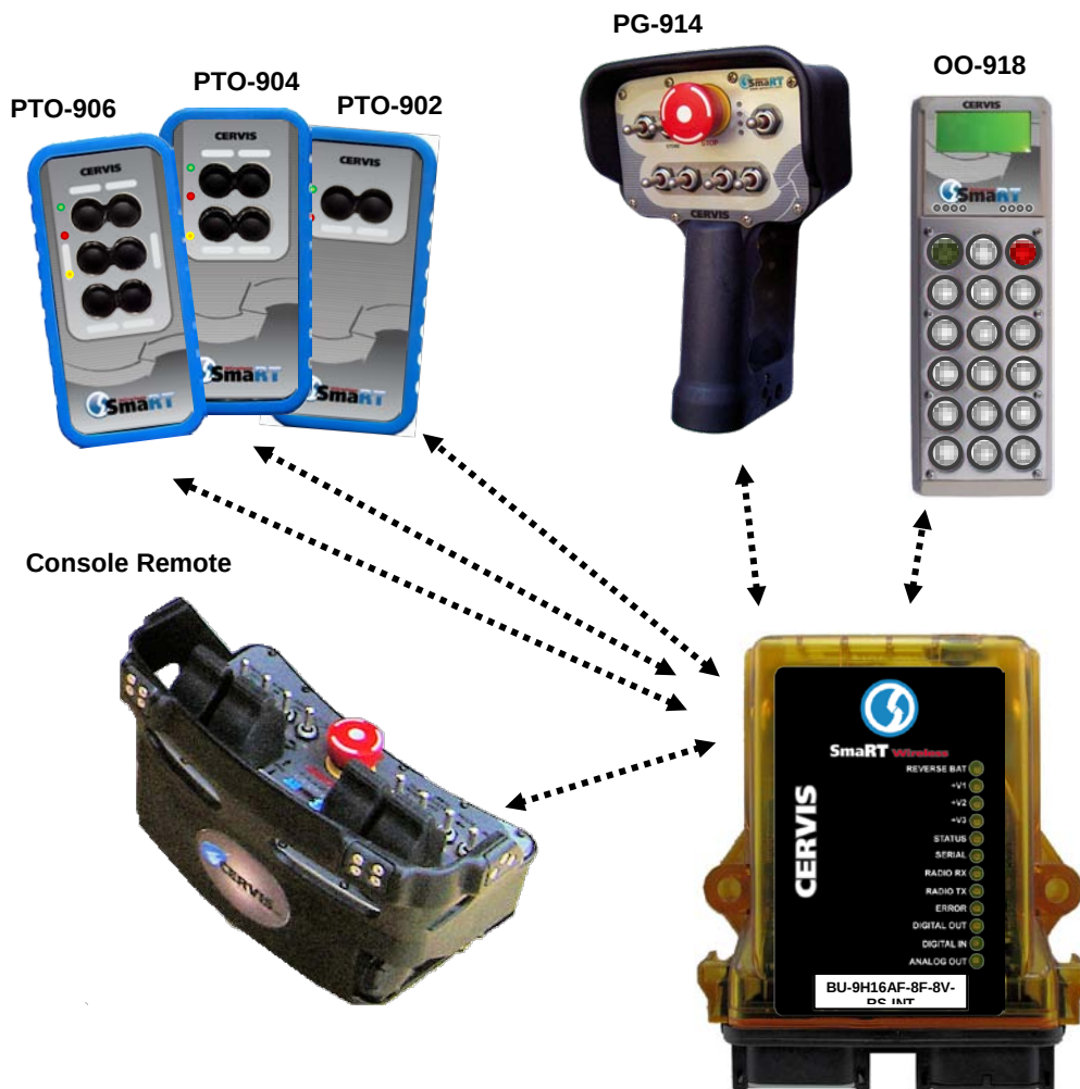
Figure 2. SmaRT BU-9H16AF-8F-8V-RS with SmaRT Remote Control Units
