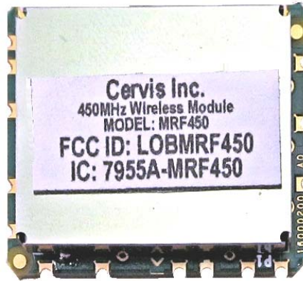
Figure 3. MRF450 RTM, Front Side with Shield and Label.
