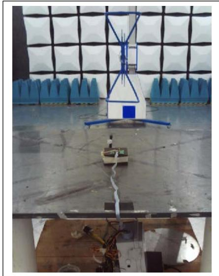
**Radiated Spurious Emissions, Greater than 1 GHz**
