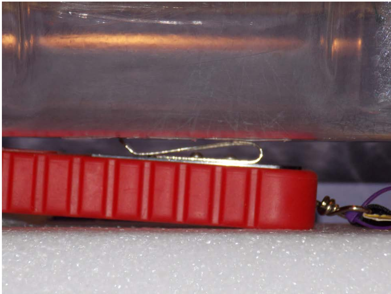
Test Position Belt Clip Main Antenna 0 mm Gap
