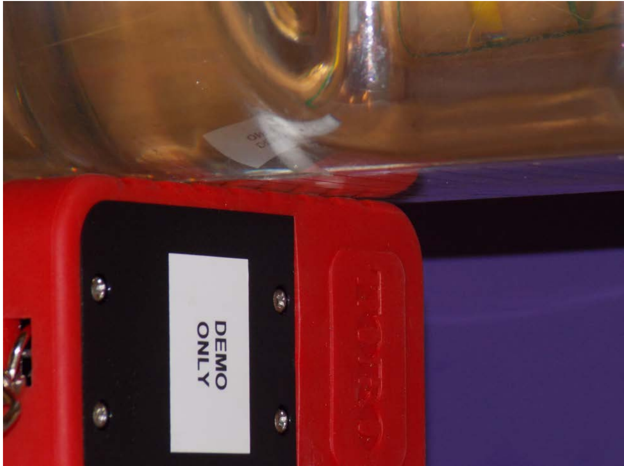
Test Position Side D Main Antenna 0 mm Gap
