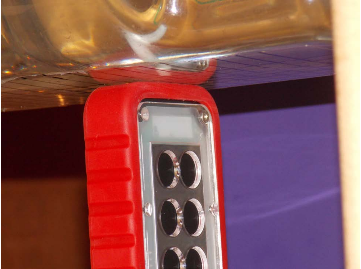
Test Position Side E Main Antenna 0 mm Gap
