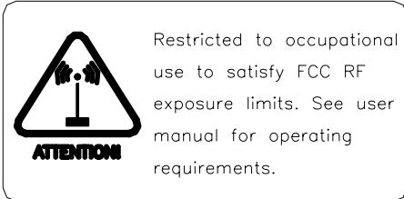
The RF Exposure Label should be affixed in the vehicle beside the mobile radio control head. The label should be in the direct view of the Repeater operator. The label is supplied with the Mobexcom P25 DVR Repeater.
