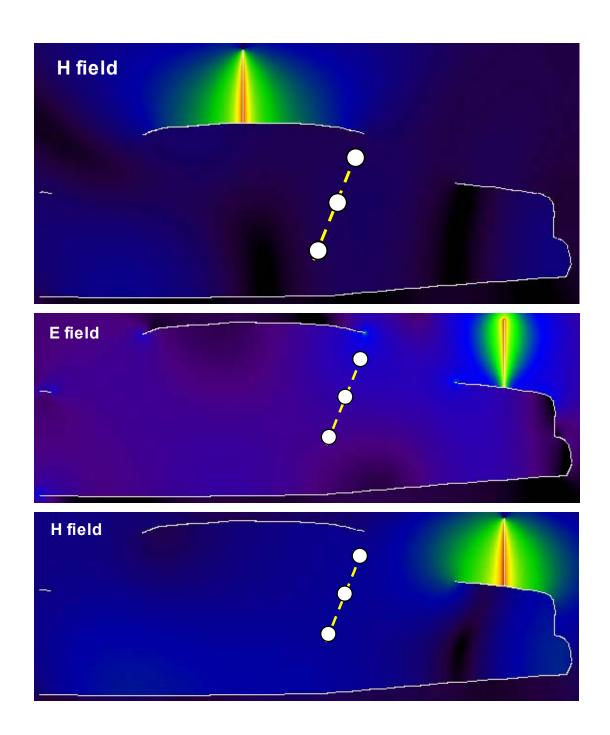
The other four pictures below additionally show the qualitative E and H filed distributions in a vertical plane across the width of the car, crossing the center of the passenger's head. Also in this case, the first two pictures correspond to the roof-mount antenna configuration, while the last two pictures correspond to the trunk-mount antenna configuration.
