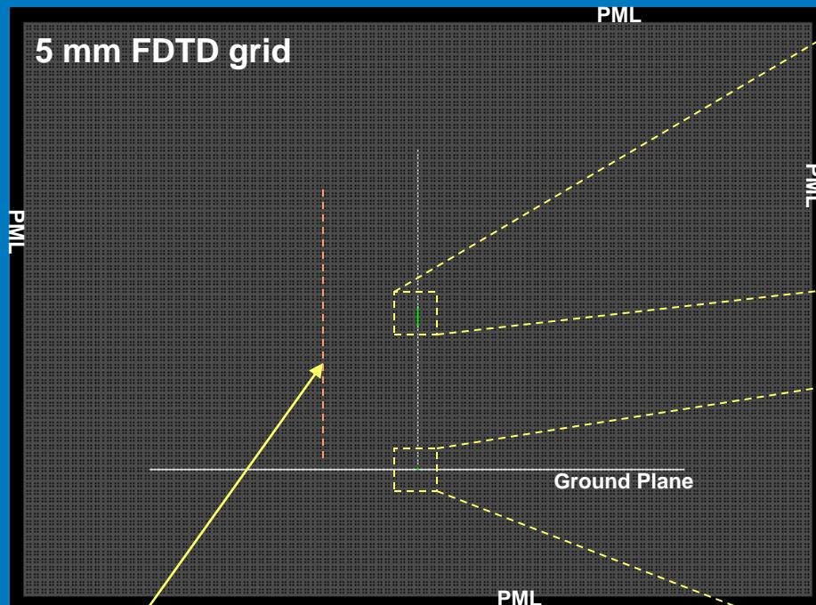
Lines at 20 cm from antenna along which the simulated and measured field values were compared
