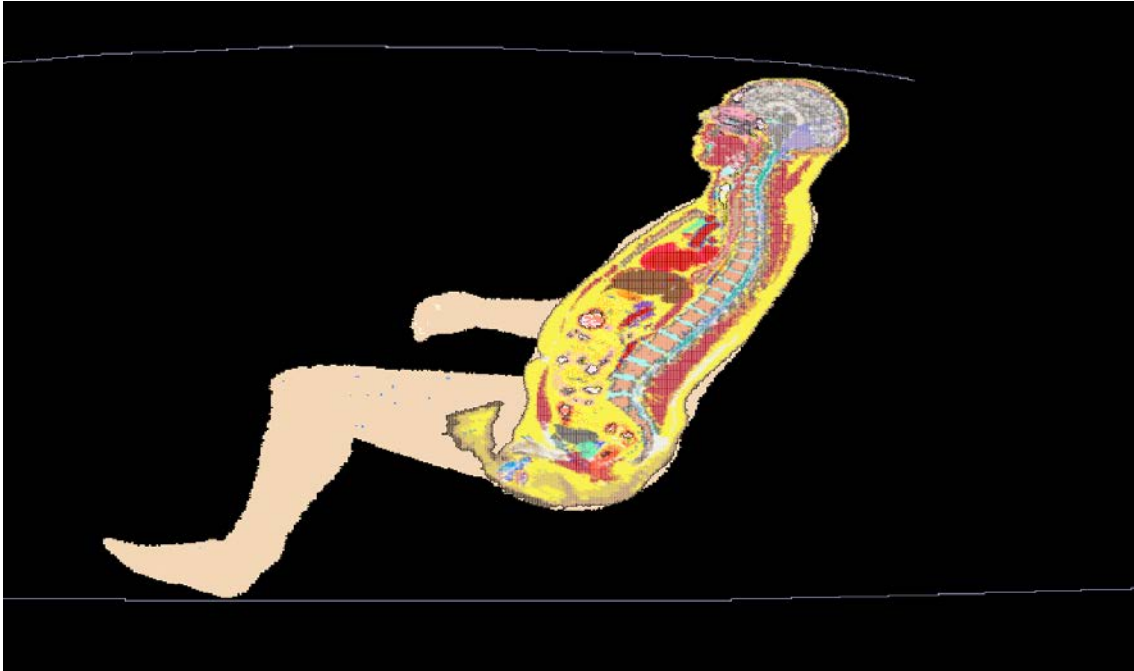
Figure 2: Passenger model exposed to a trunk-mount antenna: XFDTD geometry.
