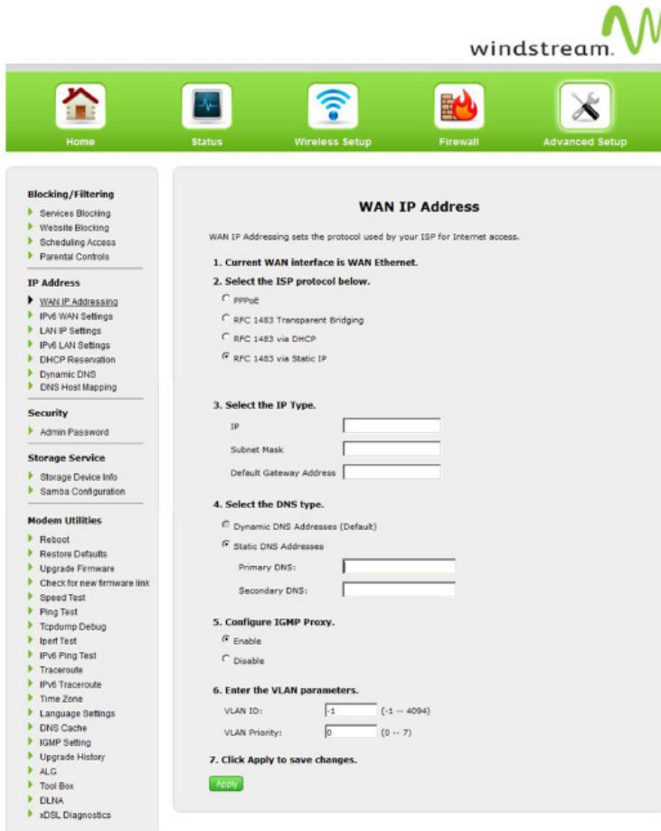
The screenshot shows the Windstream T3280 Gateway's web-based configuration interface. At the top, there is a navigation bar with icons for Home, Status, Wireless Setup, Firewall, and Advanced Setup. The Home icon is selected. The main content area is titled "WAN IP Address". It contains the following steps:
