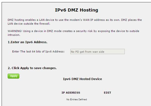
**Caution!** A DMZ host is not protected by the firewall and may be vulnerable to attack. Designating a DMZ host may also put other computers in the local network at risk. When designating a DMZ host, consider the security implications and protect it if necessary.
