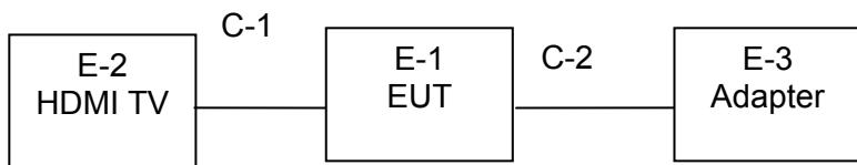
Radiated Emission Test
