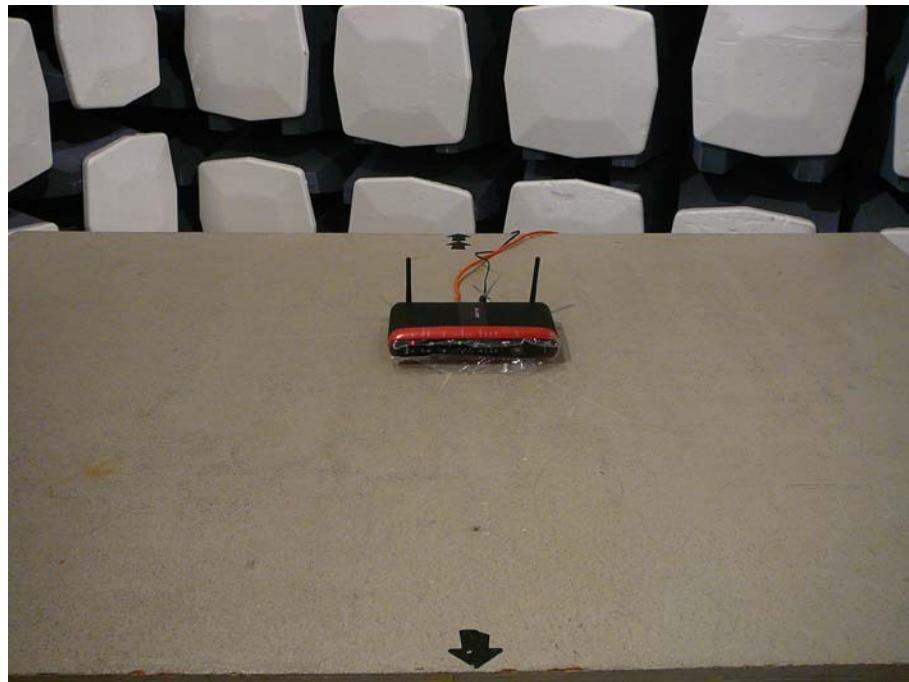
**14.6 Radiated Emissions – Rear View (Above 1 GHz)**
