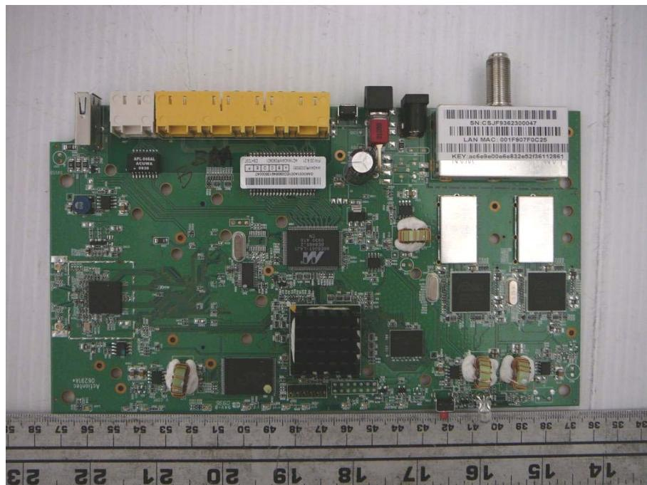
**15.9 Main Board Top View (without Shielding)**
