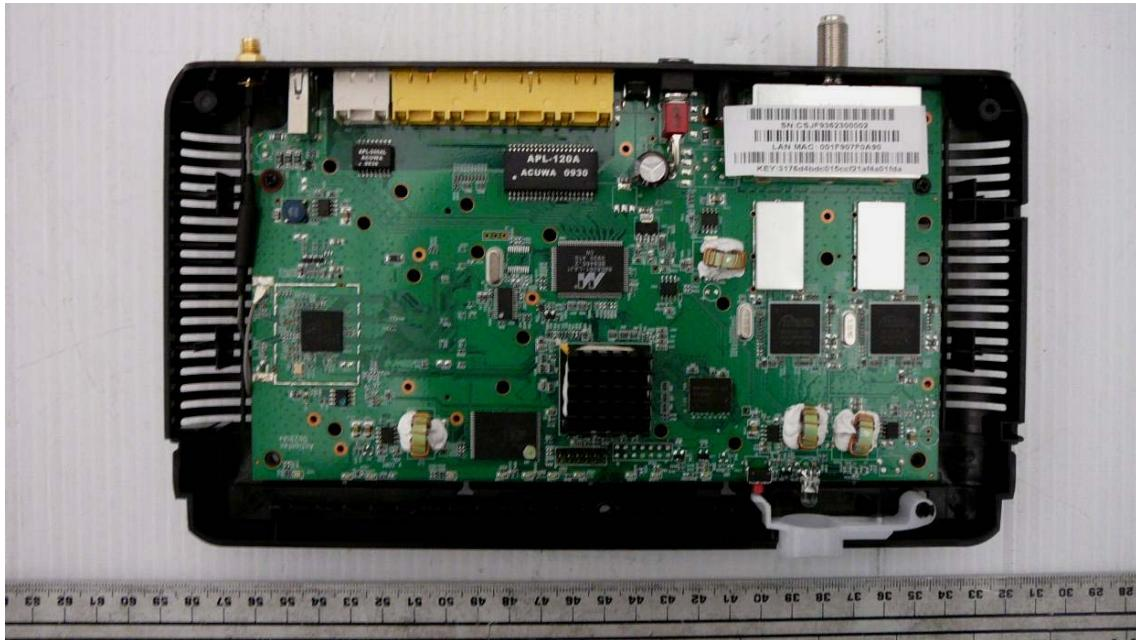
**15.6 EUT- Main Board Top View-(RF with Shielding)**
